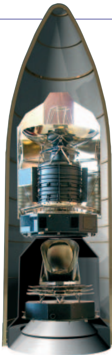
Herschel (top) and Planck will be launched jointly by the most powerful version of Ariane-5 into a direct transfer orbit to L2
